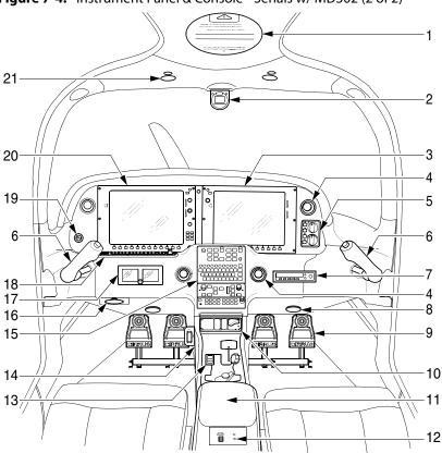
Figure 7-4: Instrument Panel & Console - Serials w/ MD302 (2 of 2)
