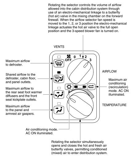
**NOTE:** Illustration depicts settings for Emergency Procedures <u>Smoke and Fume Elimination</u>. If source of smoke and fume is firewall forward, turn Airflow Selector OFF.
