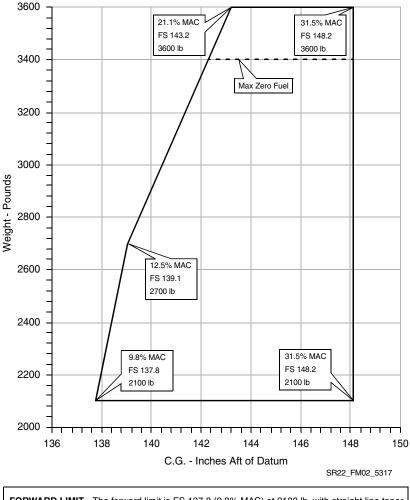
FORWARD LIMIT - The forward limit is FS 137.8 (9.8% MAC) at 2100 lb, with straight line taper to FS 139.1 (12.5% MAC) at 2700 lb, to FS 143.2 (21.1% MAC) at 3600 lb. AFT LIMIT - The aft limit is FS 148.2 (31.5% MAC) at all weights from 2100 lb to 3600 lb.
