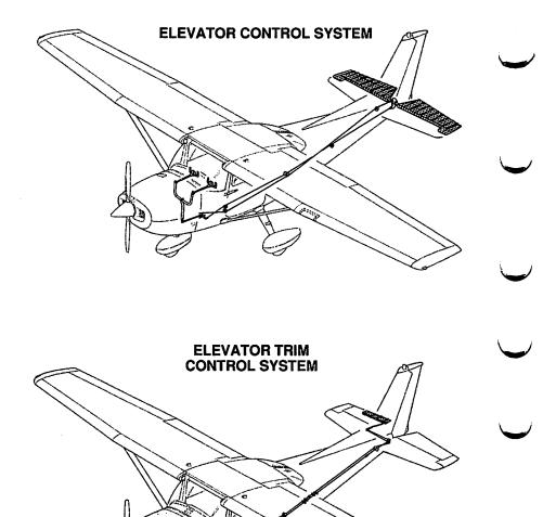
Figure 7-1. Flight Control and Trim Systems (Sheet 2 of 2)
