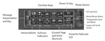
Figure 1 - GNX 375 Control and Display Layout
