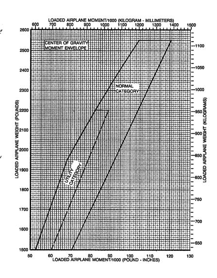
Figure 6-7. Center of Gravity Moment Envelope
