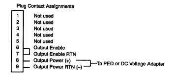
Figure 3. Mating Plug Wiring
